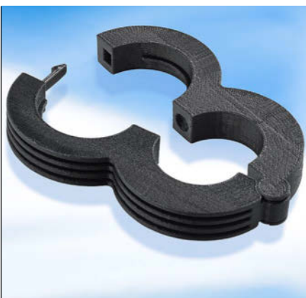
Hose clamp with closure | Material: PA or PC | Layer height: 0.27 mm | Build time: approx. 4.5 hours
