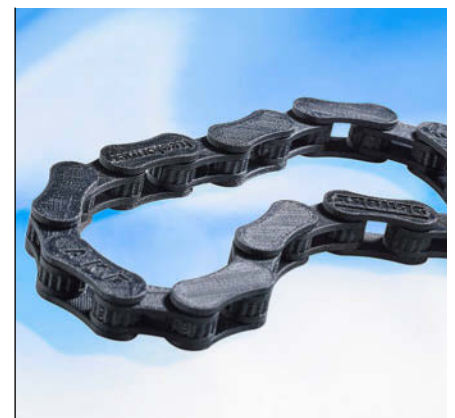
Chain produced as a component without an assembly step | Material: ABS | Layer height: 0.21 mm | Build time: approx. 8 hours
