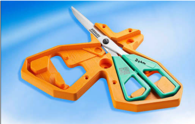
Jig for holding office scissors | Material: ABS | Layer height: 0.27 mm | Build time: approx. 19 hours
